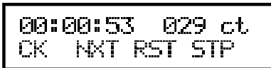
Figure 25 MCA display in running mode. The STP button will stop the MCA. The optional CK mode is shown.
