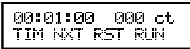
Figure 24 MCA display in stopped mode. The RUN button will start the MCA.
